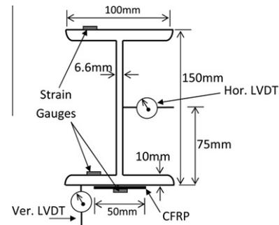
**Fig. 2.** Dimensions of steel I-section and locations of strain gauges and LVDT.
