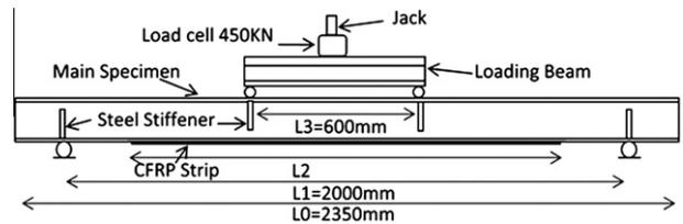
**Fig. 1.** Test setup and dimensions of steel beams.
