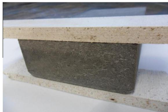
Fig. 1. Glass fibre reinforced rigid PUF and MgO Corp Board (CM-11-A007).
