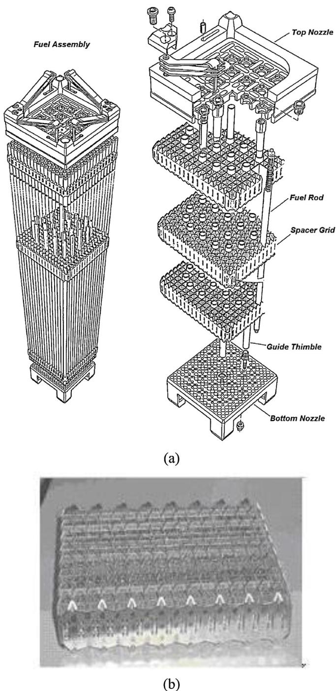
**Fig. 1.** Fuel assembly structure: (a) the fuel assembly and its components and (b) geometry of the spacer grid.
