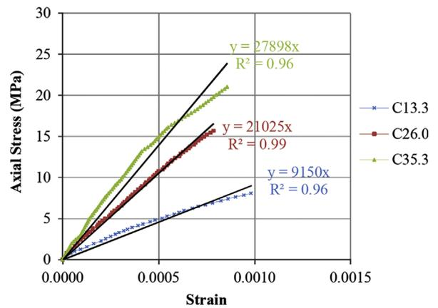
**Fig. 2.** Modulus of elasticity results for concrete specimens.
