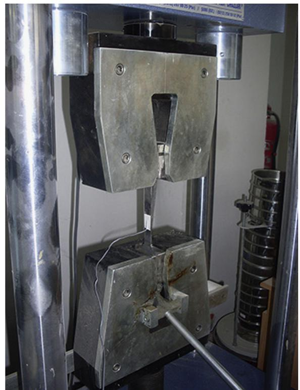
**Fig. 3.** Steel tension coupon test equipment.
