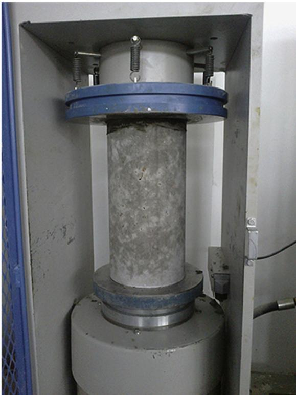
**Fig. 1.** Concrete compression test equipment.
