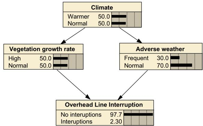
Fig. 1. Simple example of Bayesian network modelling the probability for overhead line interruptions.
