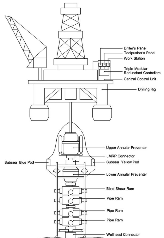
Fig. 1. Typical architecture of a subsea BOP system.
