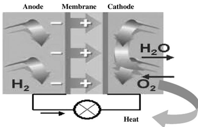
Fig. 1. Schematic diagram of a PEM fuel cell.
