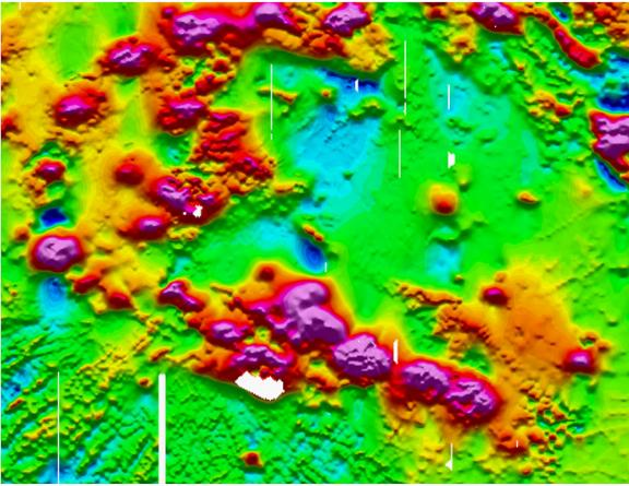
Fig. 1. Magnetic data with multiple porphyry style mineralisation. Courtesy of Barrick Gold of Australia Ltd.
