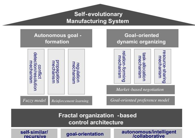
Fig. 1. Embodiment framework of a self-evolutionary manufacturing system. Shin et al. (2009a).
