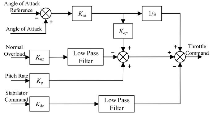
Fig. 2. The block diagram of the APCS.
