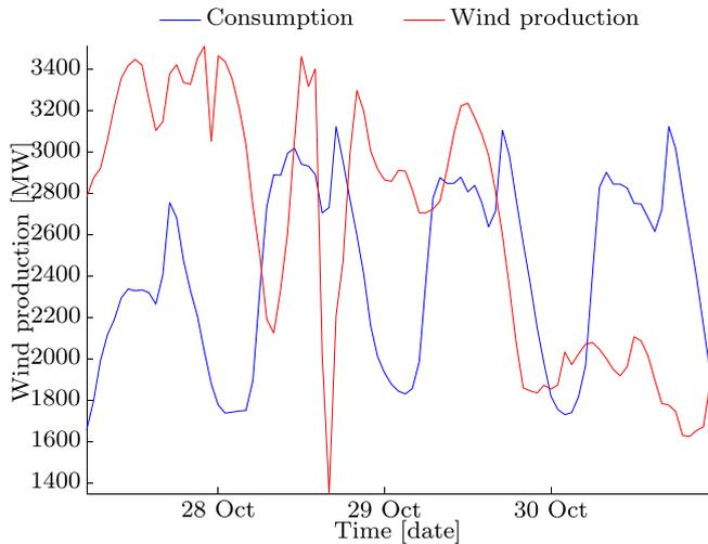
**Fig. 1.** Hourly consumption and wind production during 4 days in Denmark in end October, 2013. A storm hits Denmark in the afternoon on the 29th causing a large number of wind turbines to shut down resulting in a production drop of more than 2,000 MW in just 2 h.
