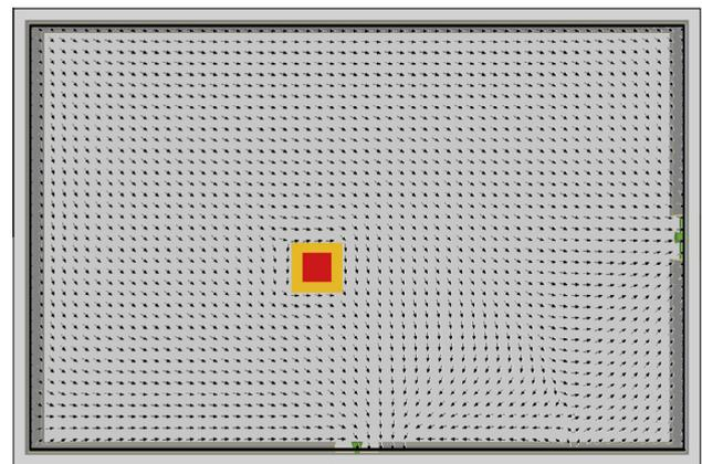
Fig. 4. The desired direction at all positions in the computational domain.
