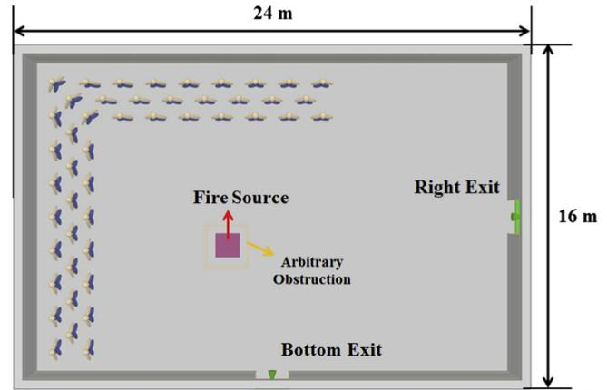
Fig. 3. The Computational domain for simulating the fire and the evacuation.
