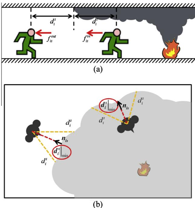
Fig. 2. The definition of the human–smoke interaction force (a), and the distance between human and the smoke boundary (b).
