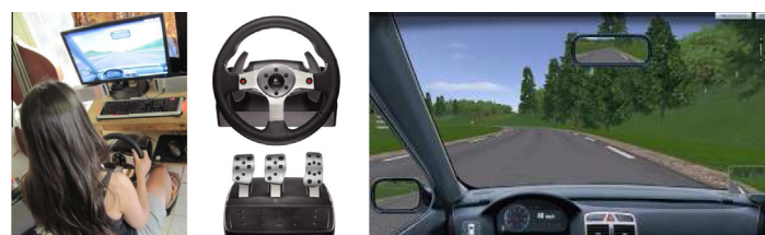
Fig. 2. The realistic prototype setup (left), the used input device used (middle) and a screen-shot of the simulator (right).
