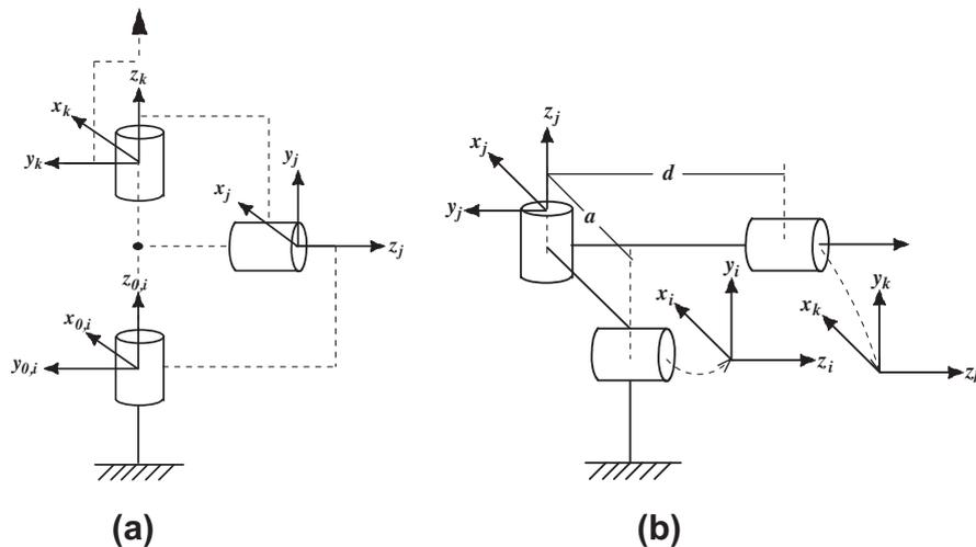
Fig. 1. The structures of (a) Euler wrist, (b) offset wrist.
