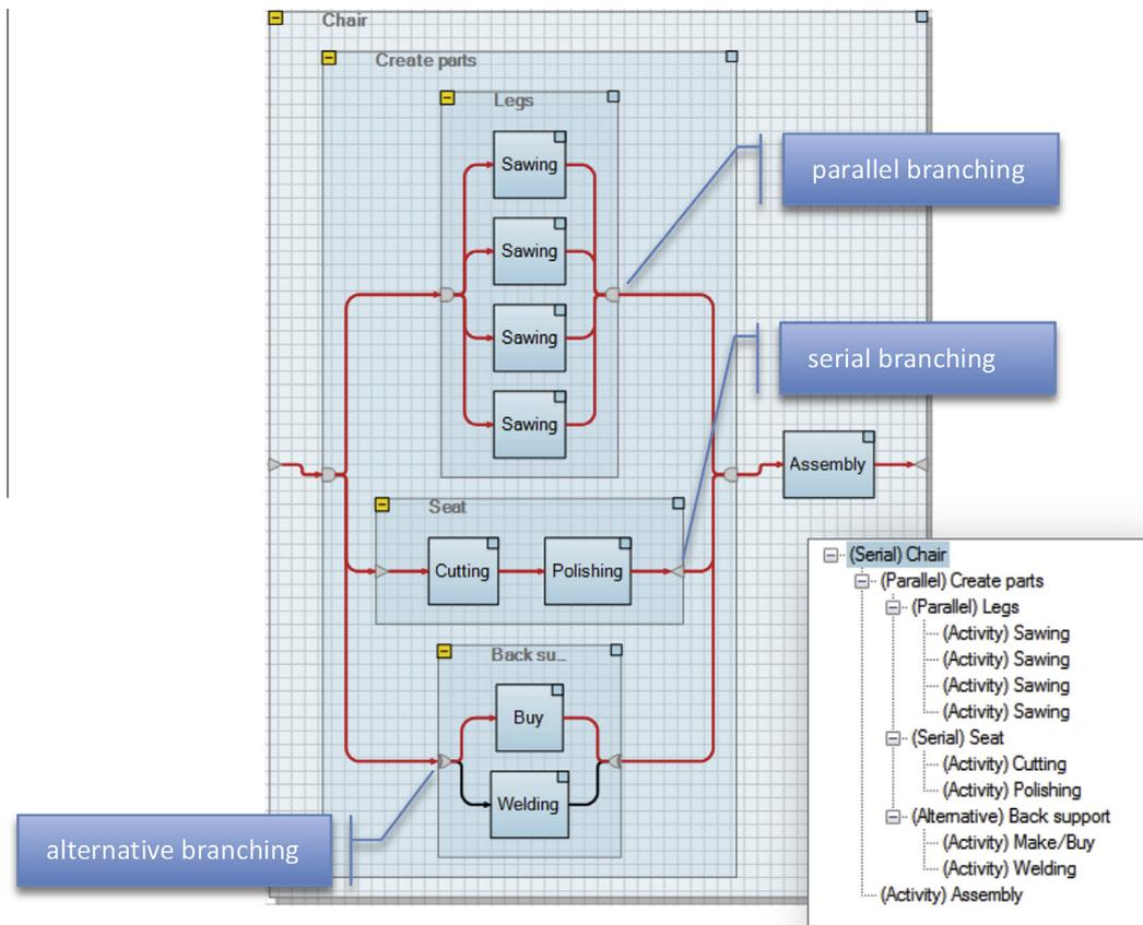
Fig. 1. Nested workflow as it is visualized in the FlowOpt Workflow Editor (from top to down there are parallel, serial, and alternative decompositions).
