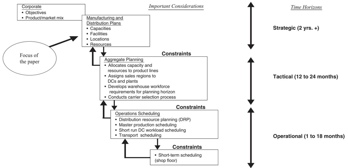
Fig. 1. The hierarchical manufacturing and distribution planning framework.
