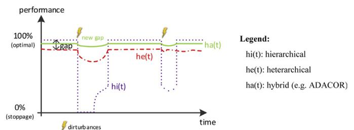
Fig. 1. Performance behaviour of different classical control structures.
