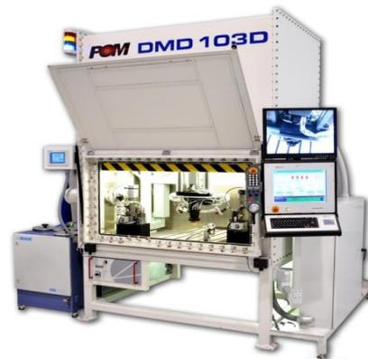
Fig. (1a): DMD machine prototype;
