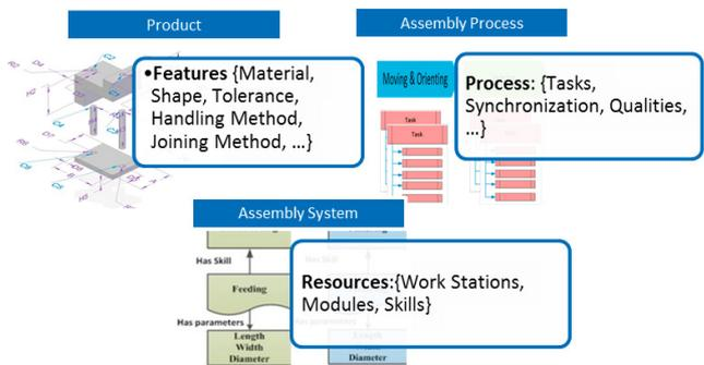
Fig. 2. Key aspects of an assembly system..
