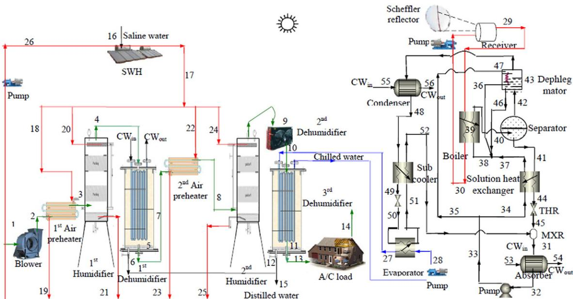
Fig. 1. Two stage desalination and cooling plant.
