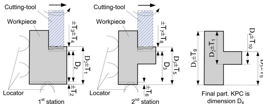
Fig. 1. Example of the influence of machining-induced variations on the tolerance allocation problem.
