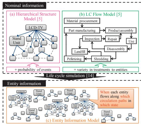
Fig. 1 Framework of a modelling method for LC design focusing on entities throughout product life cycles
