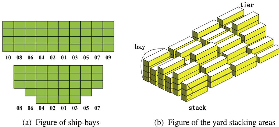
Fig. 1. Ship-bays and the corresponding yard stacking areas.
