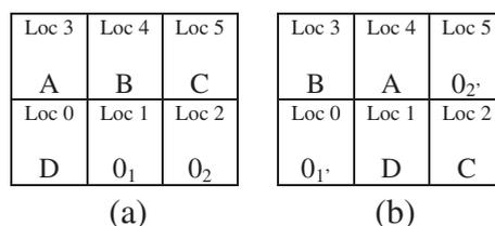
Fig. 1. The initial (a) and final (b) configurations for a sample reshuffling problem.
