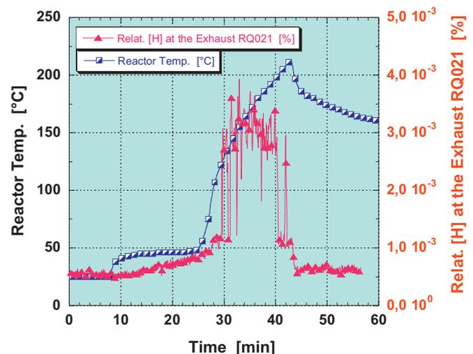
Fig. 2. Hydrogen content in the exhaust gas versus time during warming up of the reactor bed.
