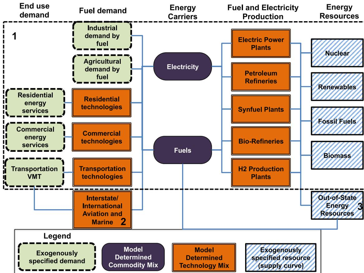
Fig. 1. Schematic representation of CA-TIMES model. The numbers refer to three categories of emissions sources: Included (sources in dashed box 1), Overall (sources 1+2), and Lifecycle (sources 1+2+3) emissions explained in Section 3.5.
