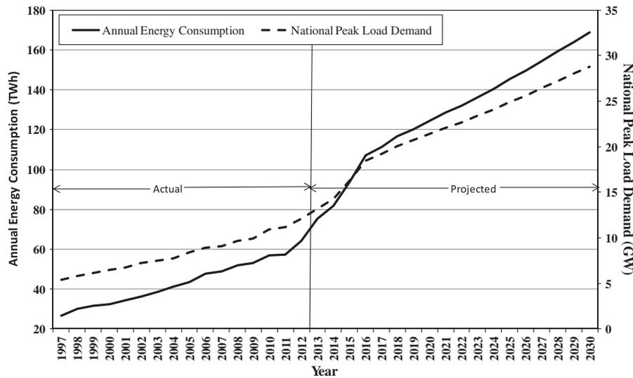
Fig. 1. Actual and projected annual energy consumption and national peak load demand from 1997 to 2030 [17,18].
