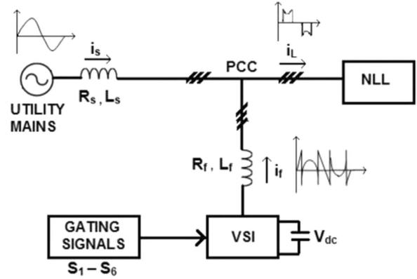
Fig. 1. Compensation principle of SAPF.
