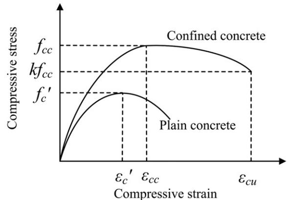
Fig. 3. Uniaxial stress–strain curve for plain and confined concrete.
