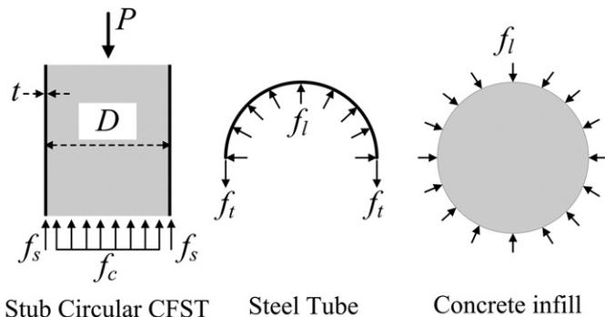
Fig. 2. Stress distribution of stub circular CFST under axial load.
