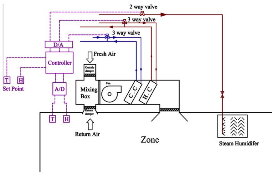
Figure 2 Schematic of control FCU with control signal.
