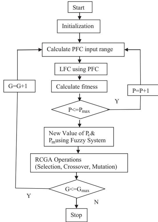
Fig. 3. Flow chart of adaptive PFC using GAF.
