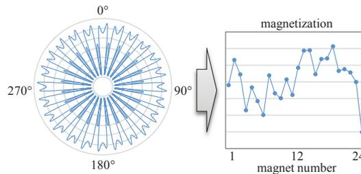
Fig. 2. Space-resolved magnetization measurement  $B(\varphi)$  of one rotor stack (left) and the resulting discrete signal  $B(k)$  (right).
