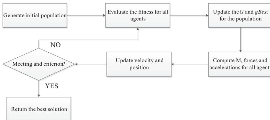
Fig. 2. The principle diagram of the PSOGSA [12].
