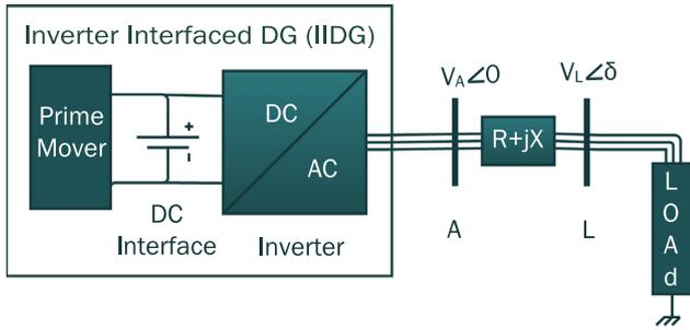
Fig. 1. DG connected with an interfaced inverter system and load.
