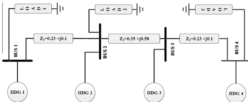
Fig. 3. An MG with four DGs and three load banks.
