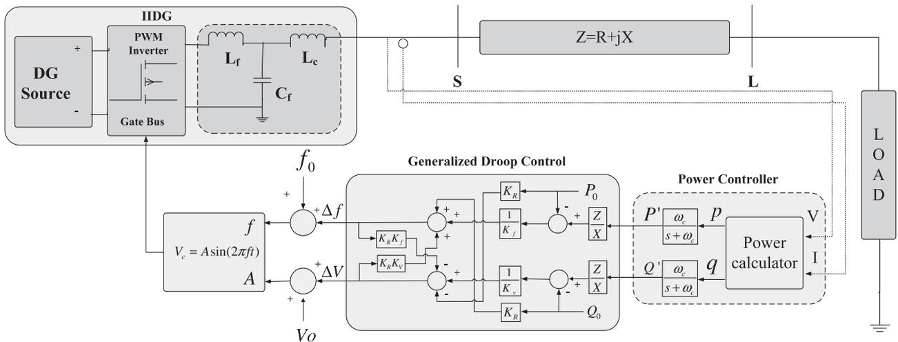
Fig. 2. Block diagram of an IIDG controlled by GDC.
