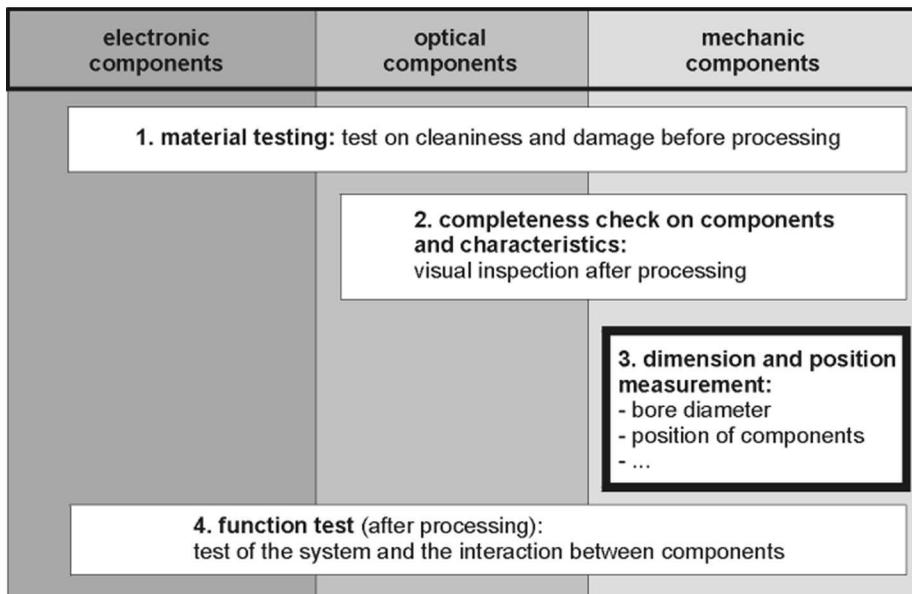
Fig. 1. Measurements tasks in the field of microtechnology.
