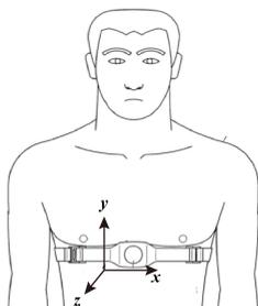
Fig. 1. Swim logger and its axis definition.
