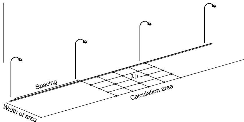
**Fig. 2.** One-sided installation.
