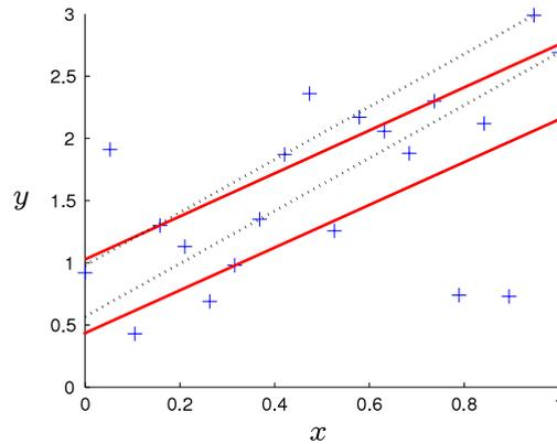
**Fig. 1.** We require 50% of the data (blue crosses) are covered by a tube. The result of the  $\nu$ -SVR (3) is illustrated by red solid lines. Black dotted lines display the optimal solution to (1). The two tubes cover the same amount of the data samples, but the distributions of the outliers are different.
