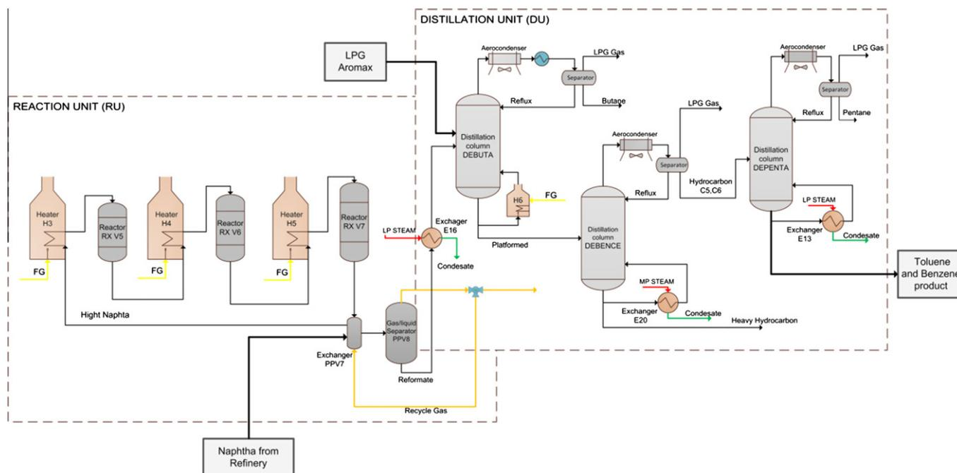
Fig. 1. Process flow diagram of the platforming unit.
