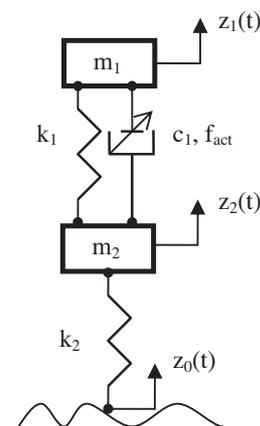
Fig. 1. Quarter car model with semi-active suspension.
