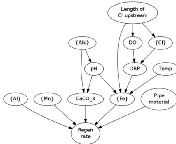
Fig. 1. Potential factors determining material accumulation rate
