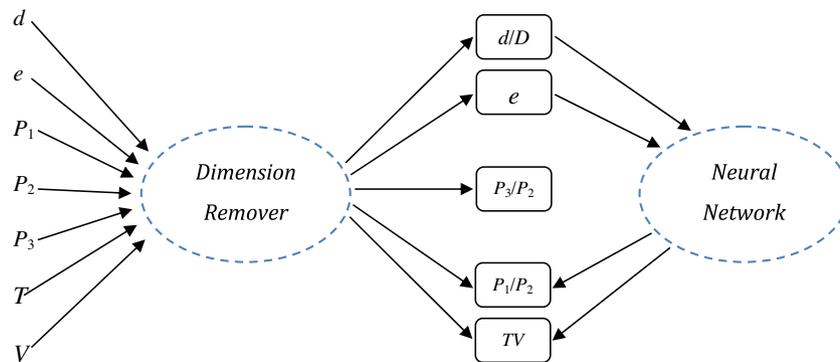
**Fig. 1.** Dimensional analysis and defining the inputs and the outputs of the ANN model.
