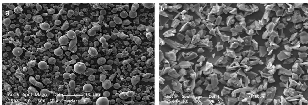
**Fig. 2.** SEM micrographs of elemental powders (a) Al and (b) SiC.
