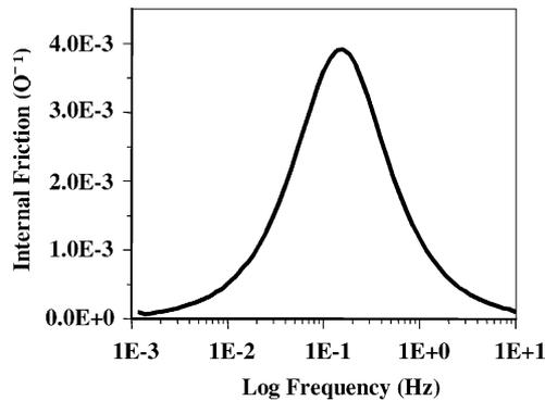
Fig. 1. Typical Snoek peak for interstitial carbon.
