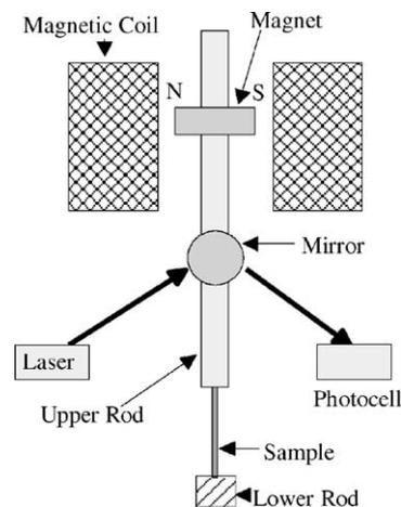
Fig. 2. Schematic diagram of the torsion pendulum.
