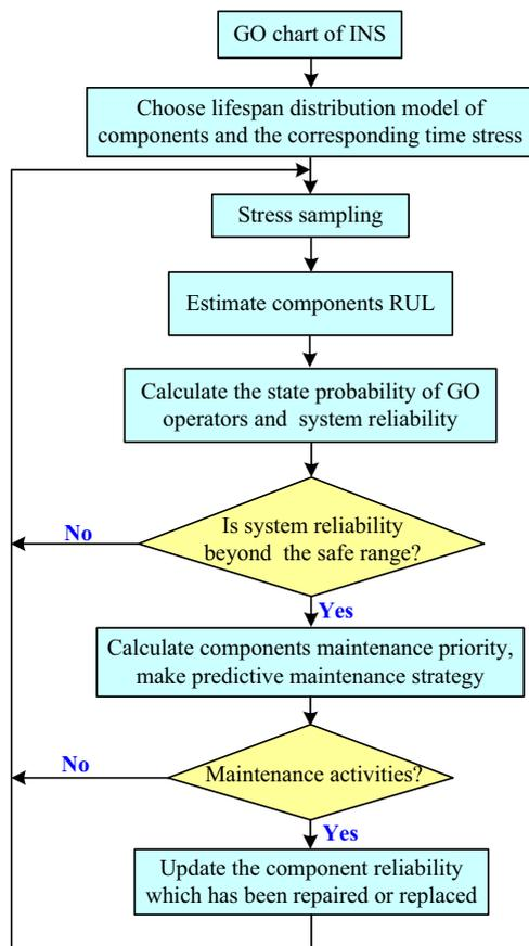
Fig. 1. The making process of reliability centered PdM for INS.
