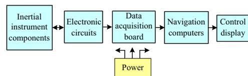
Fig. 2. Simplified logical block diagram of sample SINS.
