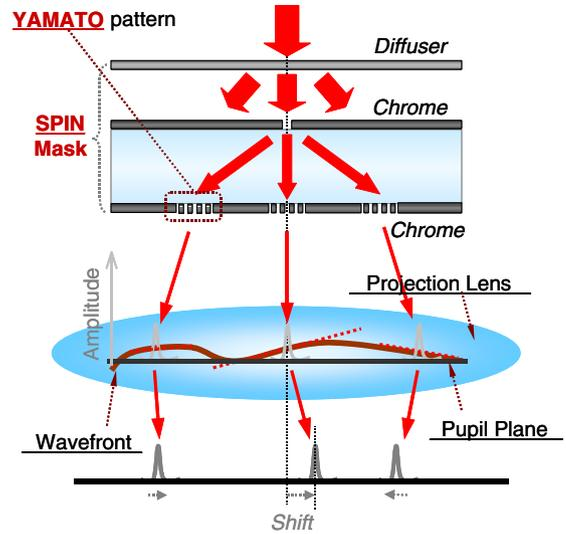
Fig. 2. Schematic diagram of SPIN method.
