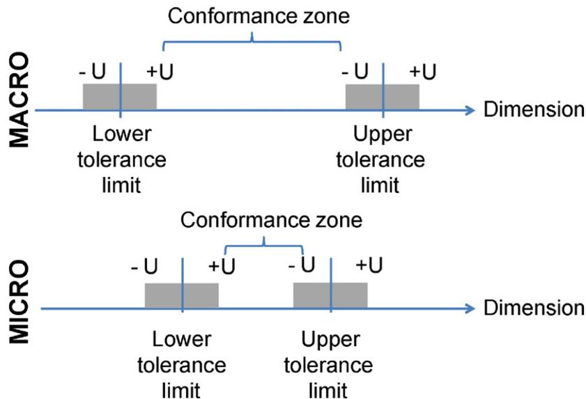
Fig. 1. Illustration of relationship between tolerance and measurement uncertainty. In this representation the measurement uncertainty was kept constant and the tolerance zone decreased.
