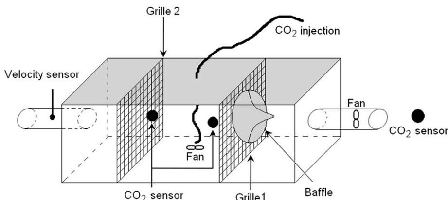
Fig. 2. Scale model apparatus.
