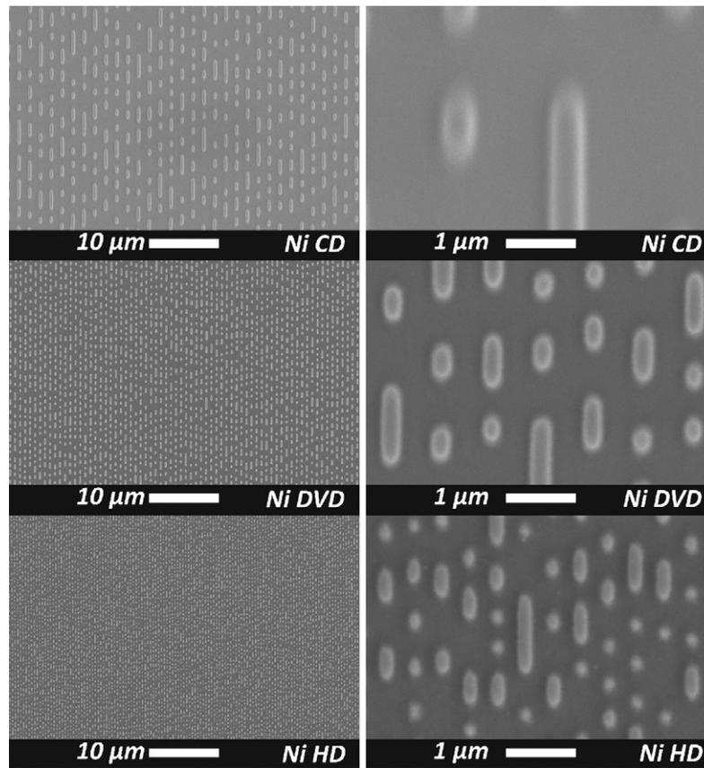
**Fig. 1.** SEM images of nickel stamper for optical discs moulding. The effect of increased data storage capacity by features miniaturization is shown on the three selected formats (CD top, DVD middle, HD-DVD bottom) both on a large surface (left) and on a detailed view (right).
