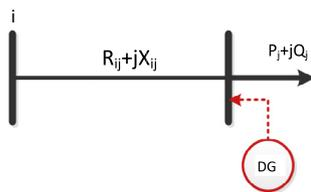
Fig. 1. Portion of a radial distribution network of  $i$ - $j$  bus.
