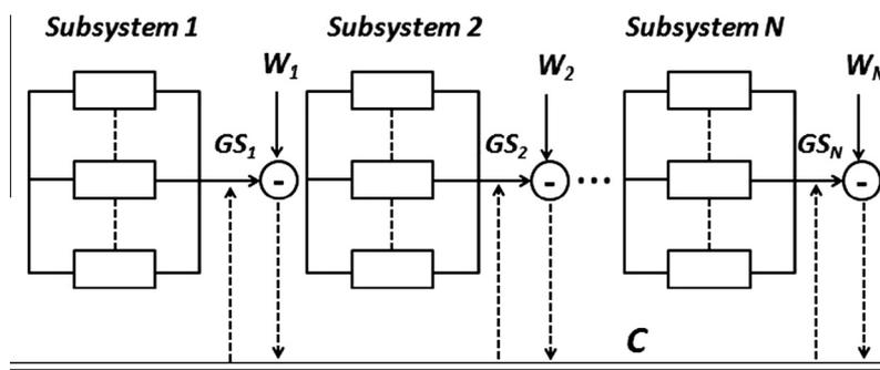
Fig. 1. Series-parallel system with common bus performance sharing.
